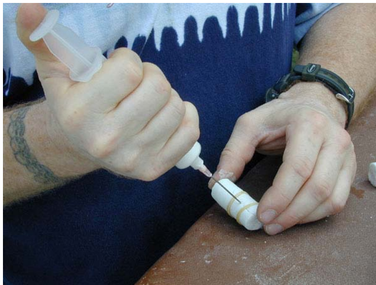
Figure 2: Preparation of DHL injected split marble cores for accelerated weathering testing (2001).
