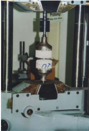
Figure 7 Direct tension test after test run
