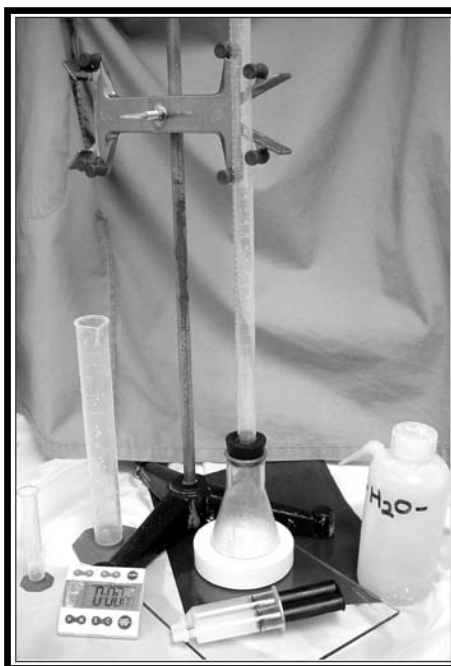
Figure 1. Author's early absorption apparatus using 2-part epoxy to attach the modified funnel to the baseplate. (ASTM STP 1432, Masonry: Opportunities for the 21st Century, 2002)
